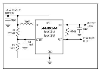
Figure 1a. MAX1833/MAX1835 Typical Operating Circuit
