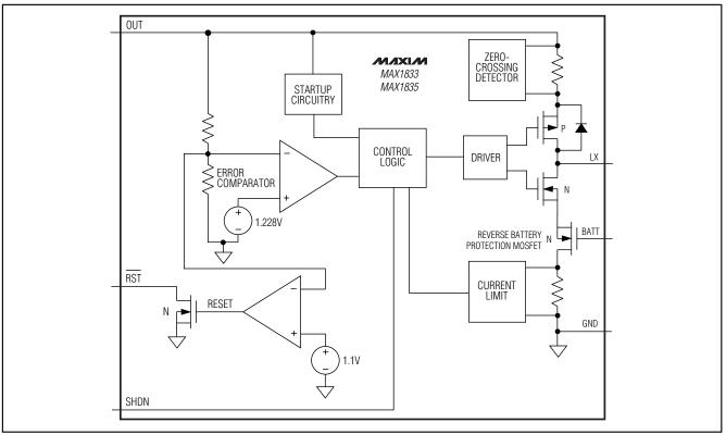
Figure 3. MAX1833/MAX1835 Simplified Functional Diagram
