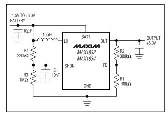
Figure 1b. MAX1832/MAX1834 Typical Operating Circuit
