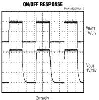
$$\label{eq:VSHDN} \begin{split} & V_{SHDN} = V_{BATT} = 2.0V, \ R_{LOAD} = 22\Omega, \\ & V_{OUT} = 3.3V \end{split}$$
