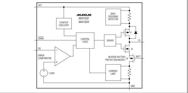
Figure 2. MAX1832/MAX1834 Simplified Functional Diagram
