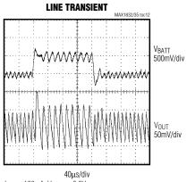
$I_{OUT} = 100$  mA,  $V_{OUT} = +3.3$ V,  $V_{BATT} = +2.0$ V TO +2.5V
