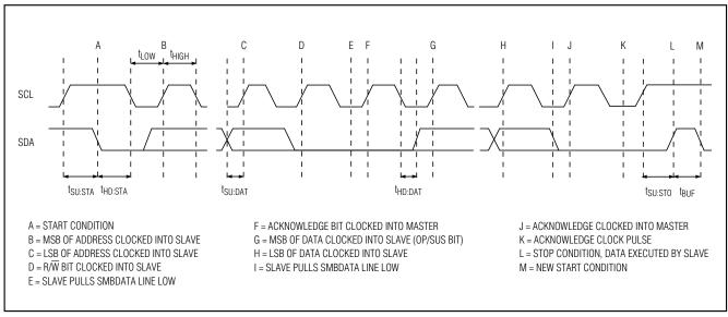
Figure 2. I<sup>2</sup>C-Compatible Serial-Interface Timing Diagram
