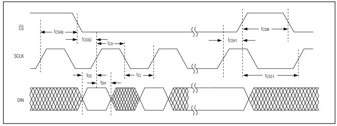
Figure 4b. Detailed Serial-Interface Timing Diagram
