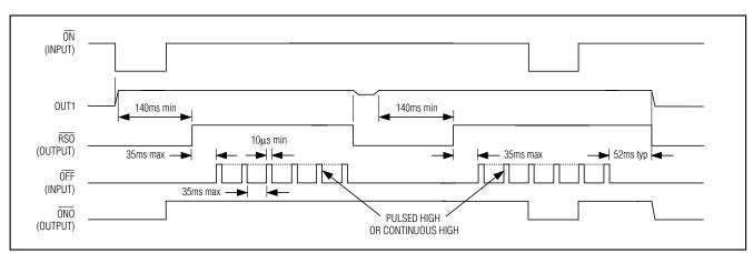
Figure 3. Push-On/Push-Off Startup and Shutdown Timing Diagram
