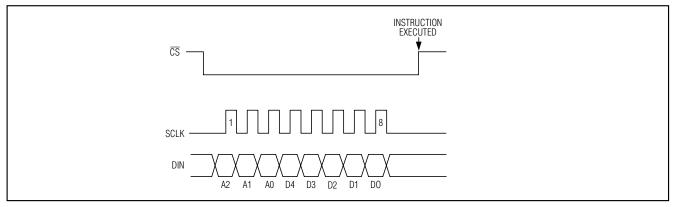
Figure 4a. Serial-Interface Timing Diagram
