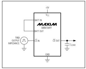
Figure 5. CE Propagation Delay Test Circuit
