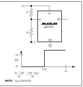
Figure 10. Monitoring a Negative Voltage
