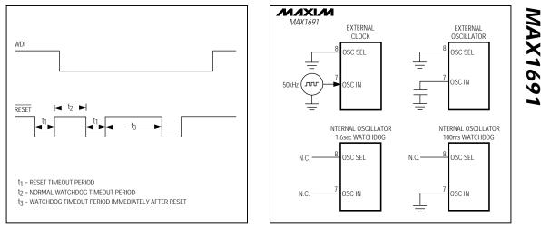
Figure 2. Watchdog Timeout Period and Reset Active Time
