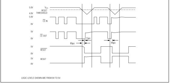
Figure 1. Reset and Chip-Enable Timing
