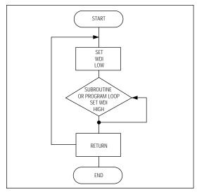
Figure 12. Watchdog Flow Diagram
