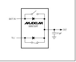
Figure 7. V<sub>CC</sub> and BATT IN to OUT Switch
