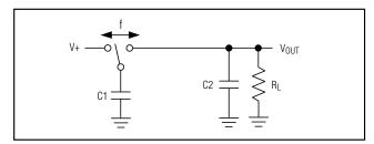
Figure 2a. Switched-Capacitor Model
