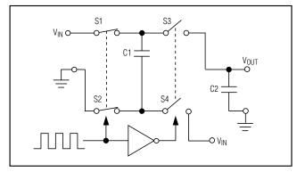
Figure 1. Simplified Functional Diagram of Ideal Voltage Doubler
