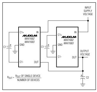
Figure 4. Paralleling Devices
