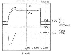
ChargingVoltage() = 0x2EE0 = 12000mV Charging Voltage(  $\gamma = 0.82EEO = 1200011V$ Charging Current( ) = 0.8FFFF = MAX VALUE ACDCIN = 18.0V, SEL = 0PEN, R1 = 0.1 $\Omega$ R2 =  $10k\Omega$ , C1 =  $68\mu$ F, C2 =  $0.1\mu$ F, C3 = 47nF  $L1 = 22\mu H$ ,  $V_{REF} = 4.096V$
