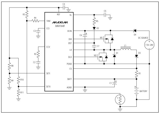
Figure 4. MAX1648 Typical Operating Circuit
