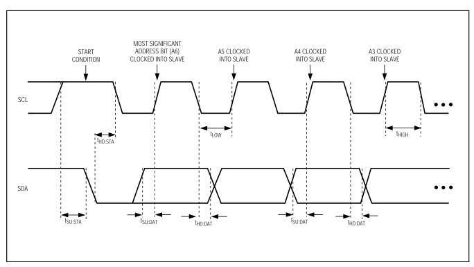
Figure 1. SMBus Serial Interface Timing—Address
