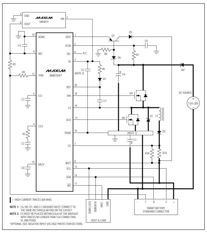
Figure 3. MAX1647 Typical Application Circuit
