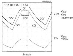
ChargingVoltage() = 0x2EE0 = 12000mV ChargingCurrent() = 0x03E8 = 1000mA ACDCIN = 18.0V, SEL = OPEN, C1 = 68µF,  $C2 = 0.1 \mu F$ , C3 = 47 n F,  $R1 = 0.1 \Omega$  $R2 = 10k\Omega$ ,  $L1 = 22\mu H$ ,  $V_{REF} = 4.096V$
