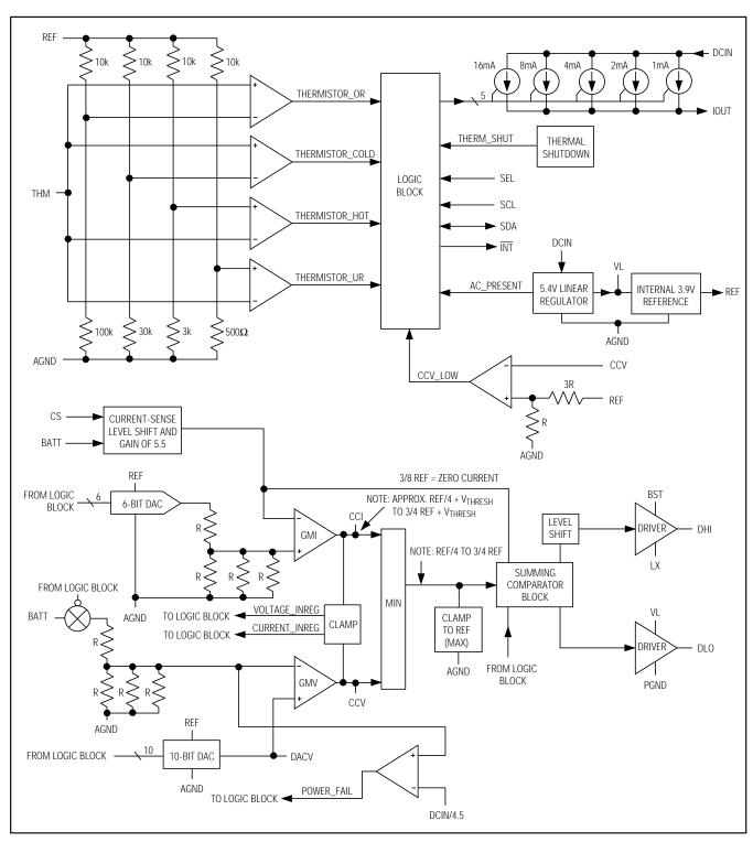
Figure 6a. MAX1647 Block Diagram
