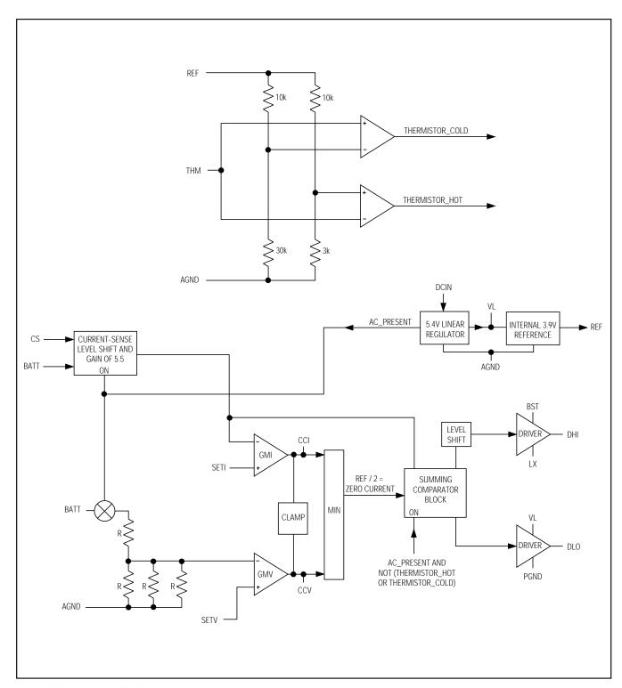
Figure 6b. MAX1648 Block Diagram
