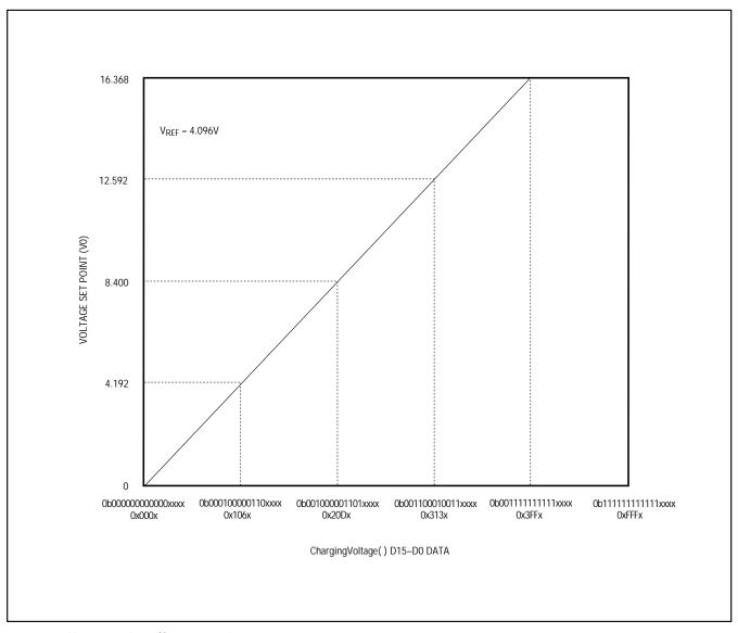
Figure 8. ChargingVoltage() Data to Voltage Mapping
