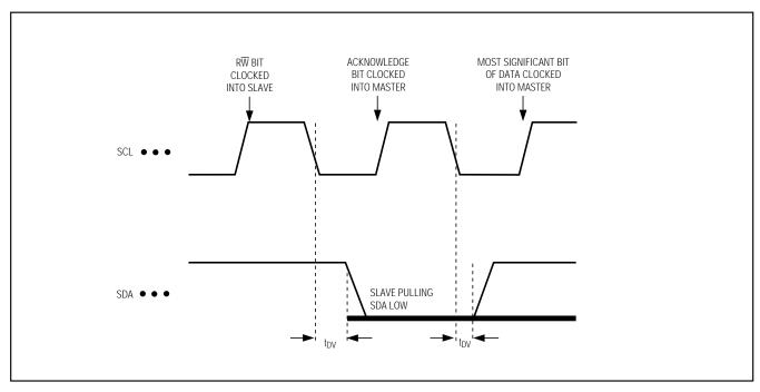
Figure 2. SMBus Serial Interface Timing—Acknowledge
