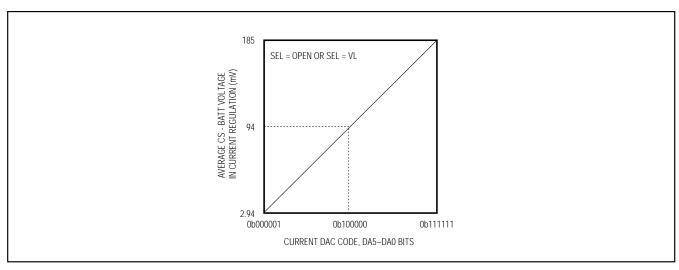
Figure 9. Average Voltage Between CS and BATT vs. Current DAC Code
