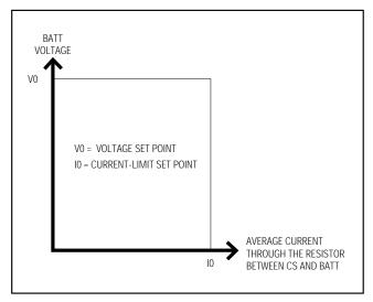
Figure 5. Output V-I Characteristic
