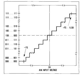
Figure 15. MAX164/167 Bipolar Transfer Function
