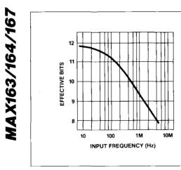
Figure 19. MAX167 Effective Bits vs. Input Frequency
