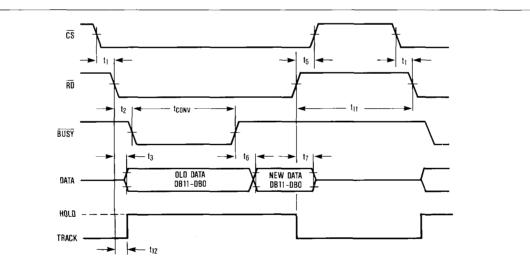
Figure 9. Slow Memory Mode, Parallel Read Timing Diagram
