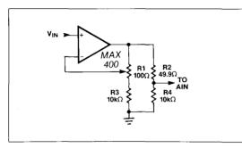
Figure 16. Trim Circuit for Gain Only ( $\pm 0.5\%$ )
