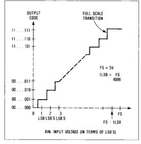
Figure 14. MAX163 Unipolar Transfer Function
