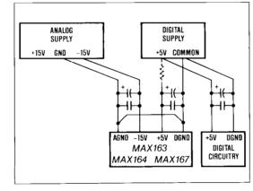
Figure 13. Power Supply Grounding Practice
