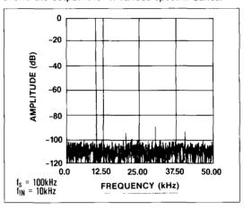
Figure 18. FFT Plot for the MAX167
