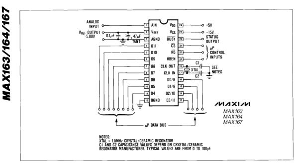
Figure 3. MAX163/164/167 Operational Diagram
