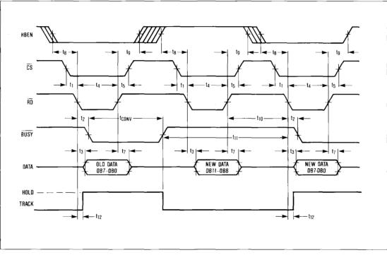
Figure 12. ROM Mode, Two Byte Read Timing Diagram
