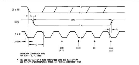
Figure 7. RD and CLK IN for Synchronous Operation
