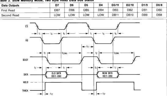
Figure 11. ROM Mode, Parallel Read Timing Diagram
