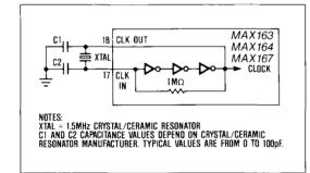
Figure 6. Internal Clock Circuit
