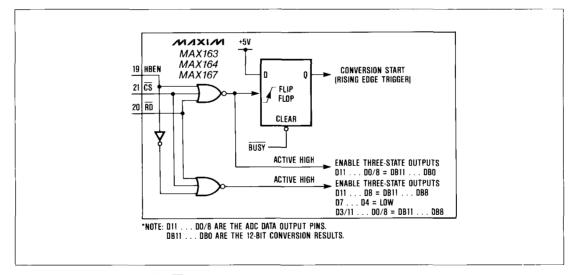
Figure 8. Logic Equivalent for RD, CS and HBEN Inputs
