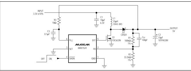
Figure 2. MAX1524 Standard Operating Circuit
