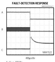
$\begin{aligned} &A:V_{OUT},\,10V/div\\ &B:V_{EXT},\,\,5V/div\\ &C:I_L,\,\,5A/div \end{aligned}$
