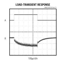
$V_{IN}$  = +3.3V,  $V_{OUT}$  = +12V,  $I_{OUT}$  = 30mA TO 120mA A :  $I_{OUT}$ , 100mA/div  $B: V_{OUT,} \ 100 mV/div, \ AC\text{-}COUPLED$
