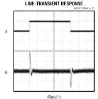
$V_{IN}$  = +3.5V TO +4.0V,  $V_{OUT}$  = +12V,  $I_{OUT}$  = 60mA A :  $V_{IN}$ , 500mV/div, AC-COUPLED B: V<sub>OUT</sub>, 10mV/div, AC-COUPLED
