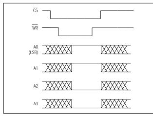
Figure 5. Programming a Four-Channel Conversion, Input Mux A
