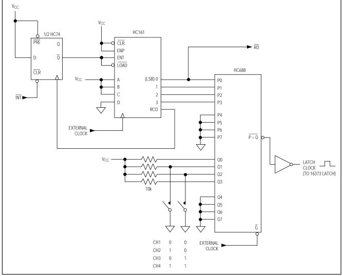
Figure 9. Output Demultiplexer Circuit
