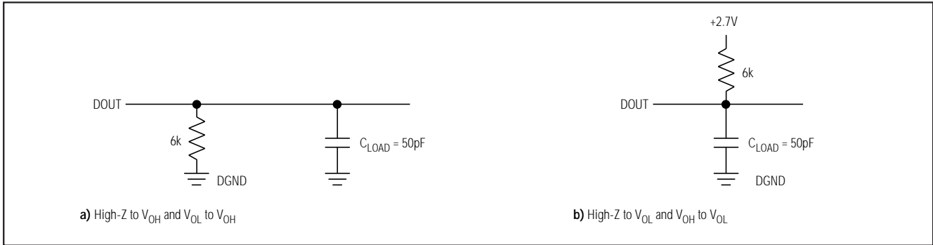
Figure 1. Load Circuits for DOUT Enable Time
