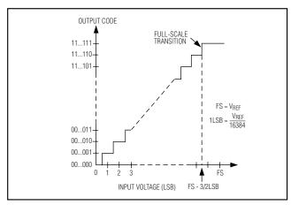
Figure 8. MAX1065/MAX1066 Transfer Function
