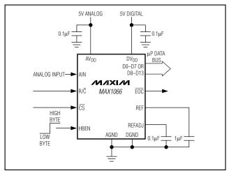
Figure 3. Typical Application Circuit for MAX1066
