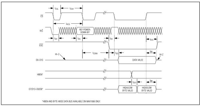
Figure 2. MAX1065/MAX1066 Timing Diagram
