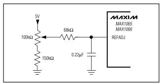
Figure 7. MAX1065/MAX1066 Reference Adjust Circuit
