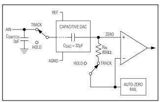
Figure 4. Equivalent Input Circuit
