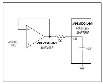
Figure 9. MAX1065/MAX1066 Fast Settling Input Buffer
