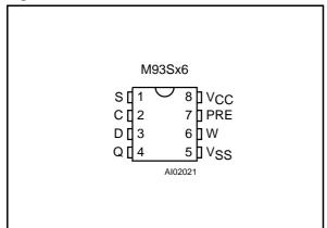
Figure 2B. SO Pin Connections
