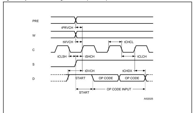
Figure 4. Synchronous Timing, Start and Op-Code Input
