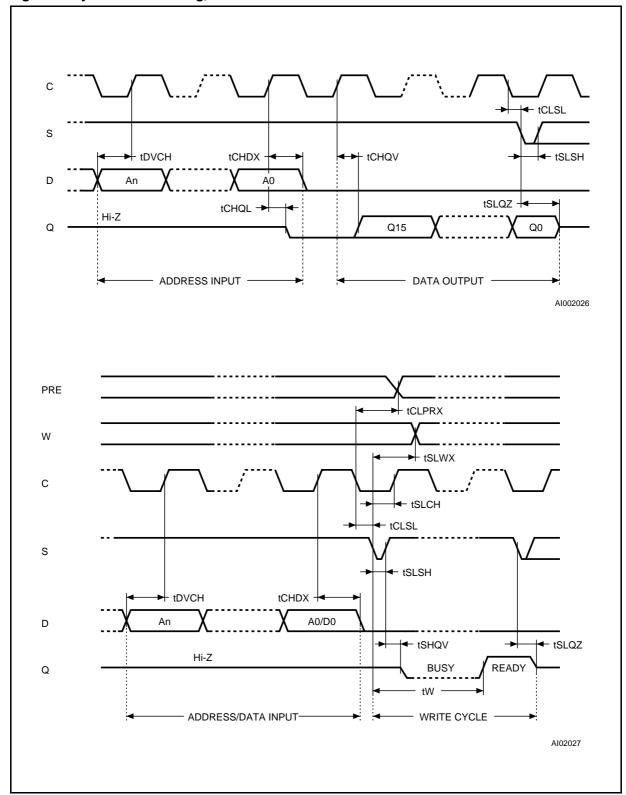
Figure 5. Synchronous Timing, Read or Write
