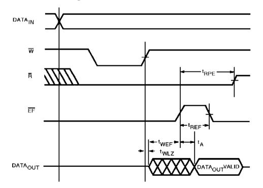
Figure 18. Write Data Flow - Through Mode.
