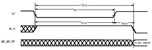
**Notes :** 23.  $\overline{EF}$ ,  $\overline{FF}$  and  $\overline{HF}$  may change status during Retransmit, but flags will be valid at  $t_{RTC}$ .
