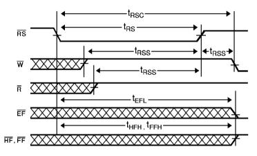
**Notes :** 1.  $\overline{\text{EF}}$ ,  $\overline{\text{FF}}$  and  $\overline{\text{HF}}$  may change status during reset, but flags will be valid at t<sub>RSC</sub>. 2.  $\overline{\text{W}}$  and  $\overline{\text{R}} = \text{V}_{\text{IH}}$  around the rising edge of RS.
