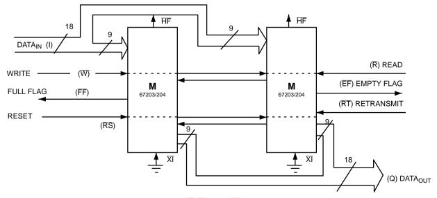
Note: 3. Flag detection is accomplished by monitoring the  $\overline{FF}$ ,  $\overline{EF}$  and the  $\overline{HF}$  signals on either (any) device used in the width expansion configuration. Do not connect any output control signals together.
