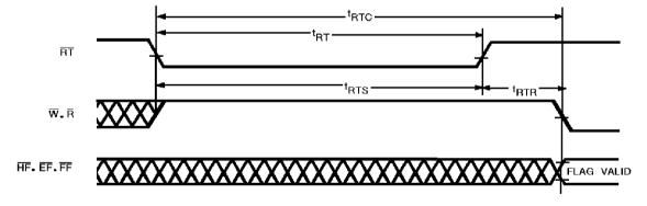
$\textbf{Note:} \quad 23. \ \overline{EF}, \overline{FF} \ \text{and} \ \overline{HF} \ \text{may change status during Retransmit, but flags will be valid at } t_{RTC}.$
