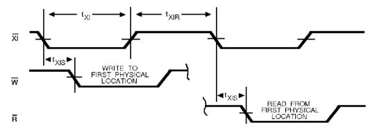
Figure 17. Read Data Flow - Through Mode.
