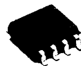
Outline 8P2S-A(FP) 1.27mm pitch 225mil SOP (4.4mmx5.0mmx1.5mm)
