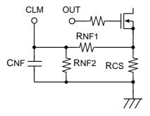
Fig.7-1 peripheral circuit of CLM
