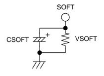
Fig.6 Method to set up duty and SOFT start function.
