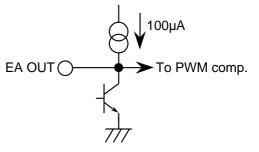
Fig.1 Circuit diagram of EAOUT terminal
