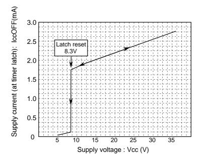
Fig.4 Supply current/voltage chracteristics (at timer latch)
