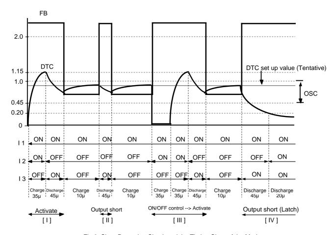
Fig.3 Short Protection Circuit and the Timing Chart of the Modes
