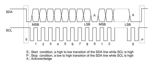
Every byte put on the SDA line must be 8-bits long . Each byte has to be followed by an acknowledge bit. Data is transferred with the most significant bit (MSB) first . The data on the SDA line must be stable during the HIGH period of the clock . The HIGH or LOW state of the data line can only change when the clock signal on the SCL line is LOW .
