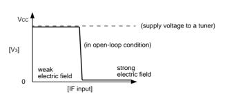
Note: Connecting a nonpolarity capacitor of 1µF between pin1 and pin 3 improves AGC operating speed.
