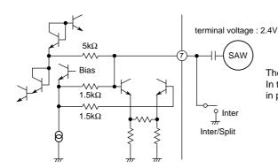
The input impedance is  $1.5k\Omega$ .
