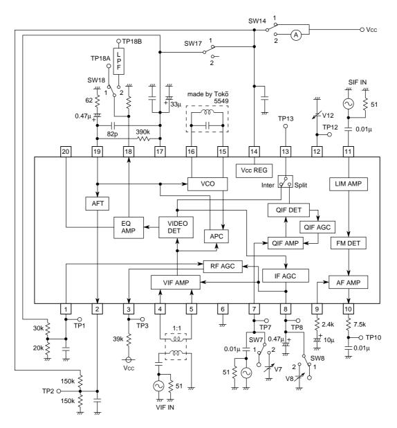
$\ast$  Capacitors without an assignment are  $0.01 \mu F.$
