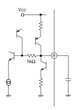
In spite of the 1-pin filter configuration, 2-pin filter characteristics are available by utilizing the dynamic AGC circuit.
