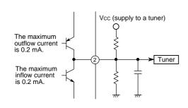
Since an AFT output is provided by a high impedance source, the detection sensitivity can be set by an external resistor.
