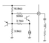
Both the external coil and capacitor determine the frequency response of EQ output.
