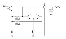
The input impedance is  $8k\Omega$ .
