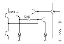
In the locked state, the cut-off frequency of the filter is adjusted effectively by an external resistor so that it will be in the range of around 30 to 200kHz.
