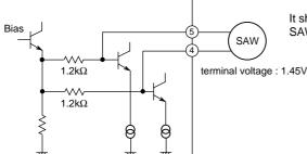
It should be designed considering careful impedance matching with the SAW filter.
