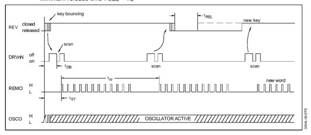
**Figure 5 :** Multiple Key-Stroke Sequence. Scan rate multiple key-stroke : t<sub>SM</sub> = 8 to 10 x T<sub>O</sub>
