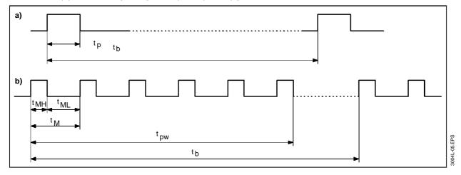
Figure 4: Single Key - Stroke Sequence. Debounce time:  $t_{DB} = 4$  to  $9 \times T_{O}$ Start time:  $t_{ST} = 5$  to  $10 \times T_{O}$ Minimum release time:  $t_{REL} = T_{O}$
