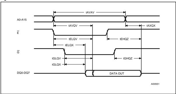
Figure 6. Read Command Waveforms
