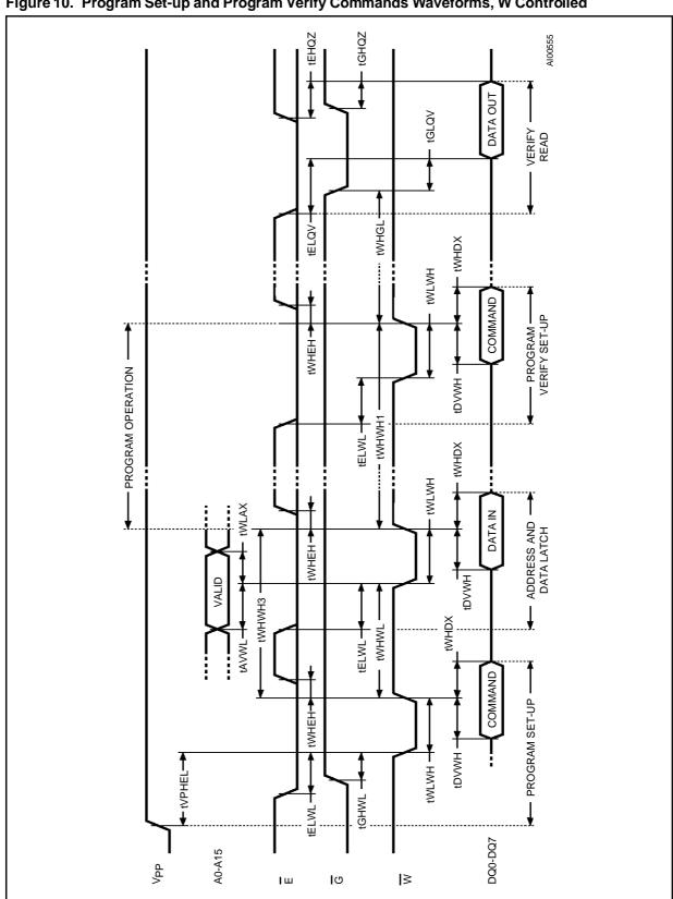
Figure 10. Program Set-up and Program Verify Commands Waveforms, W Controlled
