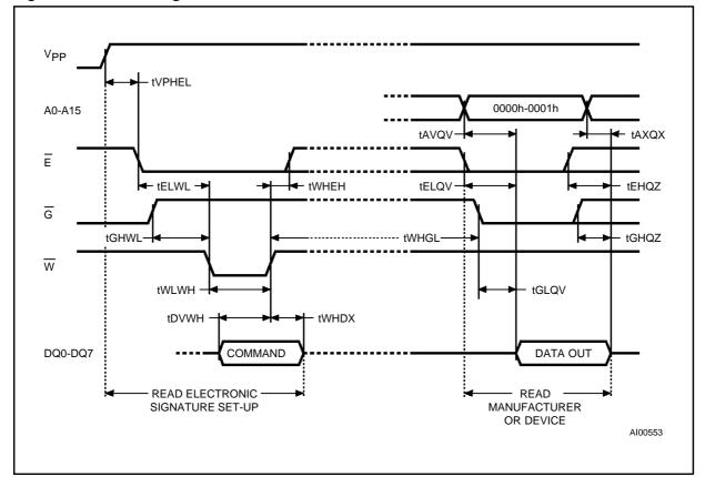
Figure 7. Electronic Signature Command Waveforms
