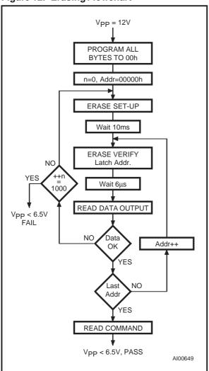
Figure 12. Erasing Flowchart
