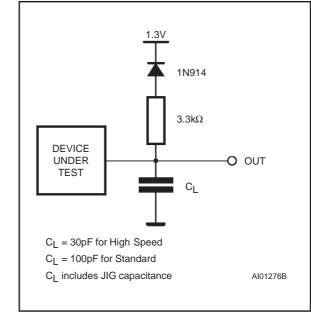
Figure 4. AC Testing Load Circuit
