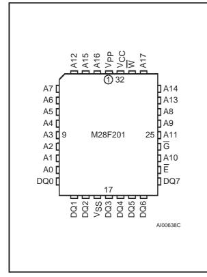
Figure 2C. TSOP Reverse Pin Connections
