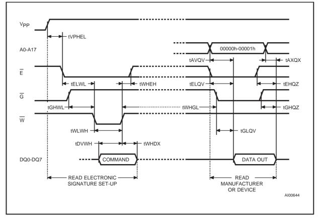
Figure 7. Electronic Signature Command Waveforms
