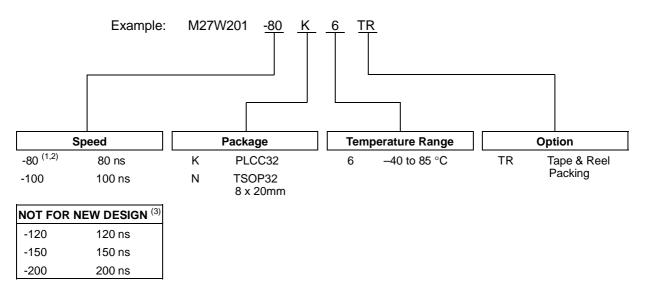
Notes: 1. High Speed, see AC Characteristics section for further information. 2. This speed also guarantees 70ns access time at  $V_{CC}$  = 3.0V to 3.6V. 3. These speeds are replaced by the 100ns.
