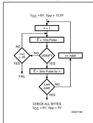
Figure 8. Fast Programming Flowchart
