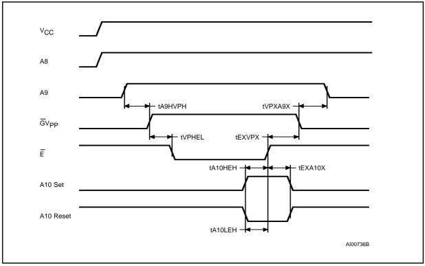
Figure 6. MARGIN MODE AC Waveform
