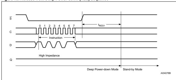
Figure 19. Release from Deep Power-down (RES) Sequence
