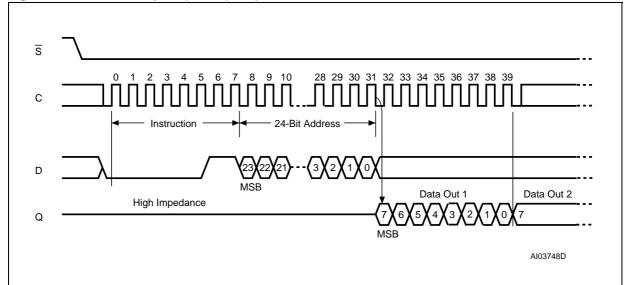
Figure 12. Read Data Bytes (READ) Sequence
