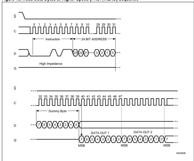
Figure 13. Read Data Bytes at Higher Speed (FAST\_READ) Sequence
