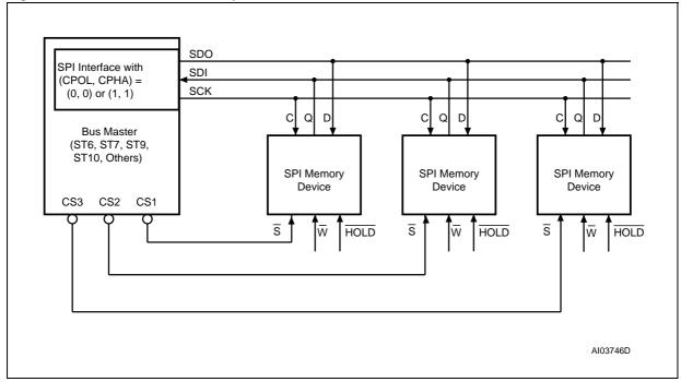
Note: 1. The Write Protect  $(\overline{W})$  and Hold  $(\overline{HOLD})$  signals should be driven, High or Low as appropriate.
