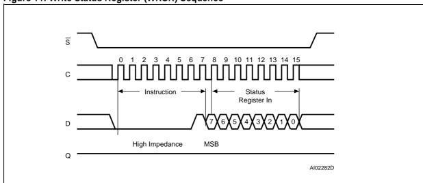
Figure 11. Write Status Register (WRSR) Sequence
