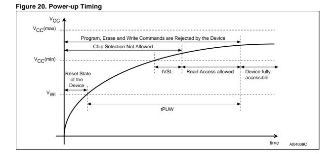
Table 7. Power-Up Timing and VWI Threshold
