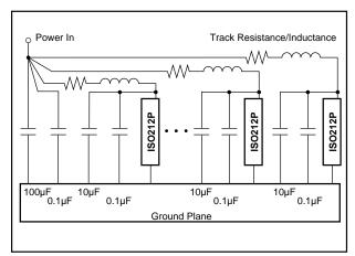
FIGURE 4. Recommended Decoupling and Power Distribution.
