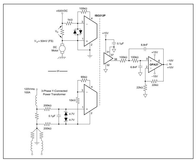
FIGURE 12. Isolated Current Monitoring Applications.
