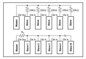
FIGURE 7. Isolating the Clk Out Node.
