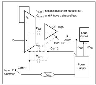
FIGURE 3. Technique for Connecting Com 1 and Com 2.
