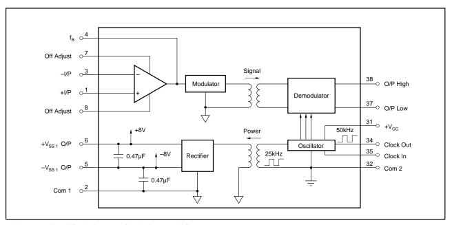
FIGURE 2. Simplified Diagram of Isolation Amplifier.
