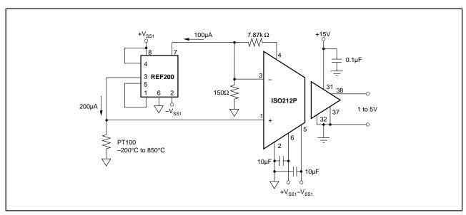
FIGURE 13. Isolated Temperature Sensing and Amplification.
