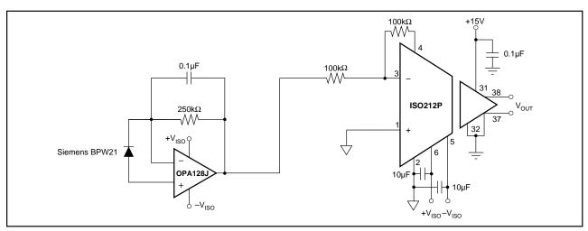
FIGURE 10. Photodiode Isolation Amplifier.
