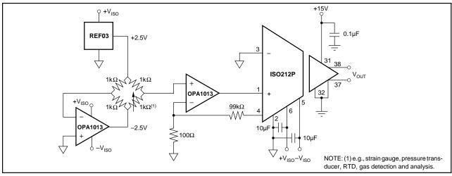
FIGURE 9. Instrument Bridge Isolation Amplifier.
