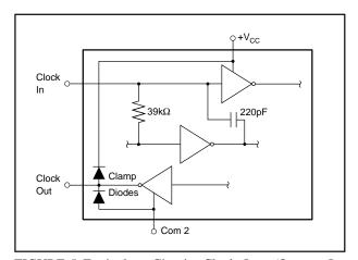
FIGURE 5. Equivalent Circuit, Clock Input/Output. Inverters are CMOS.
