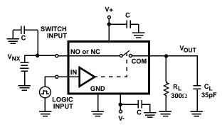
Repeat test for all switches. CL includes fixture and stray capacitance.  $$\mathsf{R}$$
