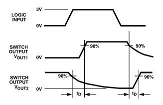
FIGURE 3A. MEASUREMENT POINTS
