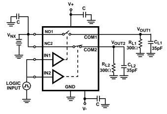
C<sub>1</sub> includes fixture and stray capacitance. Reconfigure accordingly to test SW3 and SW4.
