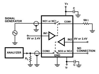
FIGURE 6. CROSSTALK TEST CIRCUIT
