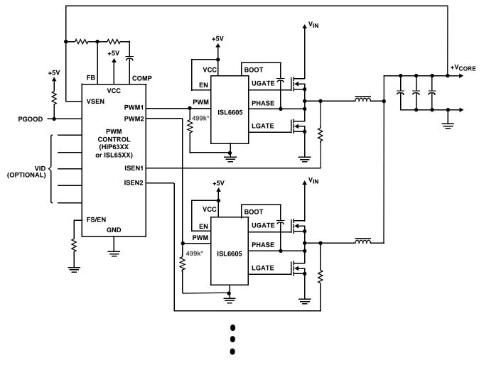
\* 499K IS USED TO PULL DOWN THE PWM INPUT TO PREVENT THE PWM FROM FALSE TRIGGERING UGATE DURING STARTUP.
