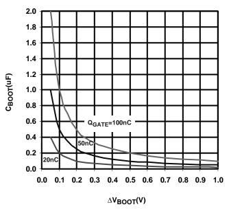
FIGURE 1. BOOTSTRAP CAPACITANCE vs. BOOT RIPPLE VOLTAGE
