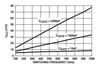
FIGURE 2. BIAS SUPPLY CURRENT vs FREQUENCY
