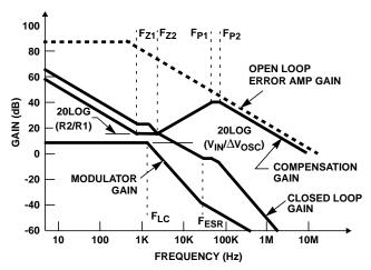
FIGURE 8. ASYMPTOTIC BODE PLOT OF CONVERTER GAIN
