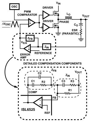
FIGURE 7. VOLTAGE - MODE BUCK CONVERTER COMPENSATION DESIGN
