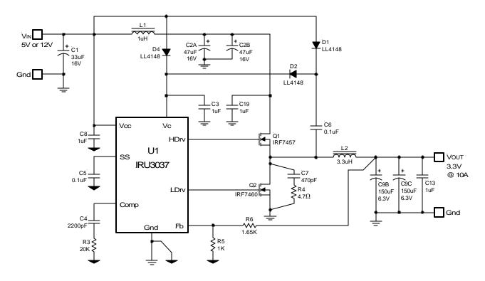
Figure 21 - Demo-board application of IRU3037.
