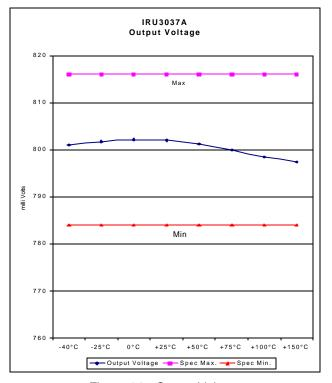
Figure 14 - Output Voltage
