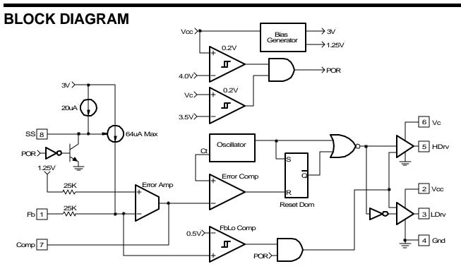
Figure 2 - Simplified block diagram of the IRU3037.
