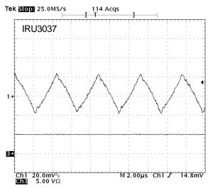
Figure 25 - 3.3V output voltage ripple @ lout=5A.
