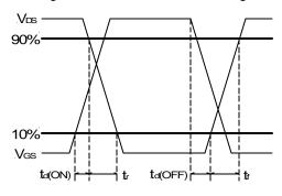
Figure 4 - Switching time waveforms.
