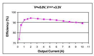
Figure 22 - Efficiency for IRU3037 Evaluation Board.
