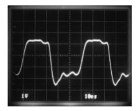
Figure 2. Driving Waveform – 20MHz
