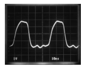
Figure 1. Receiving Waveform – 20MHz
