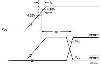
Figure 1. Timing Diagram: Power Up
