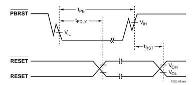
Figure 3. Timing Diagram: Pushbutton Reset
