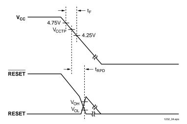
Figure 2. Timing Diagram: Power Down
