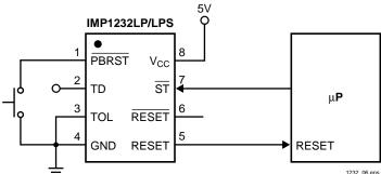
Figure 4. Application Circuit: Pushbutton Reset
