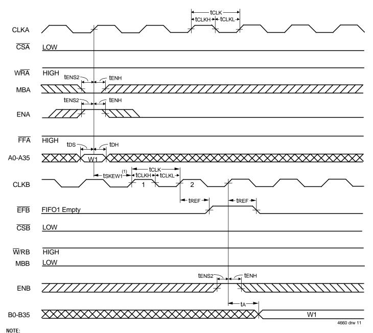
1. IskEwn is the minimum time between a rising CLKA edge and a rising CLKB edge for EFB to transition HIGH in the next CLKB cycle. If the time between the rising CLKA edge and rising CLKB edge is less than tskEwn, then the transition of EFB HIGH may occur one CLKB cycle later than shown.
