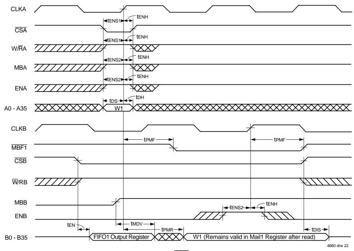
Figure 20. Timing for Mail1 Register and MBF1 Flag (IDT Standard and FWFT Modes)
