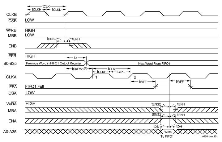
Figure 13. FFA Flag Timing and First Available Write when FIFO1 is Full (IDT Standard Mode)
