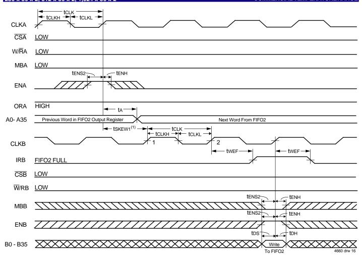
Figure 14. IRB Flag Timing and First Available Write when FIFO2 is Full (FWFT Mode)
