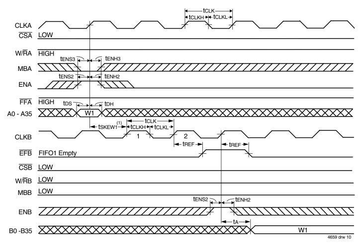
Figure 7. EFB Flag Timing and First Data Read when FIFO1 is Empty
