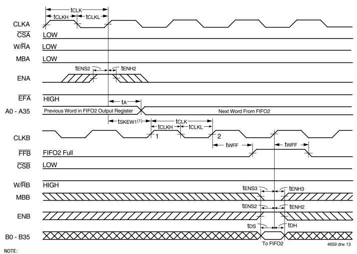
1. tskew1 is the minimum time between a rising CLKA edge and a rising CLKB edge for FFB to transition HIGH in the next CLKB cycle. If the time between the rising CLKA edge and rising CLKB edge is less than tskew1, then FFB may transition HIGH one CLKB cycle later than shown.
