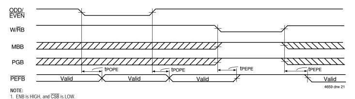
Figure 18. ODD/EVEN W/RB, MBB, and PGB to PEFB Timing
