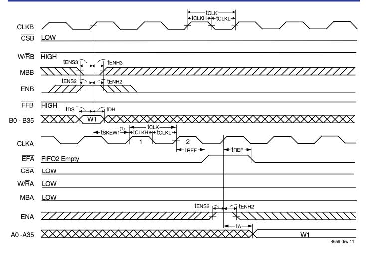
1. tskew1 is the minimum time between a rising CLKB edge and a rising CLKA edge for EFA to transition HIGH in the next CLKA cycle. If the time between the rising CLKB edge and rising CLKA edge is less than tskew1, then the transition of EFA HIGH may occur one CLKA cycle later than shown.
