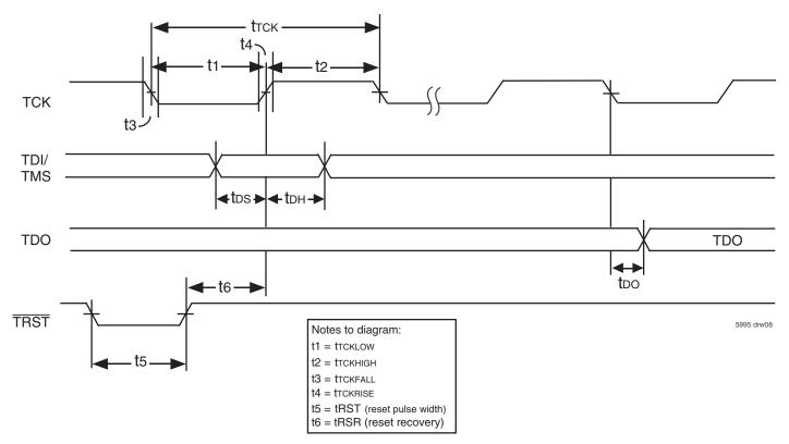
Figure 5. Standard JTAG Timing
