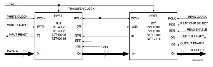
Figure 32. Block Diagram of 32,768 x 40, 65,536 x 40, 131,072 x 40, 262,144 x 40 Depth Expansion in Single Data Rate Mode
