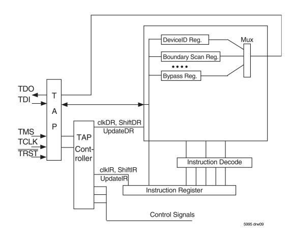
Figure 6. Boundary Scan Architecture
