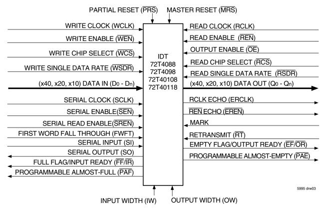
Figure 1. Single Device Configuration Signal Flow Diagram
