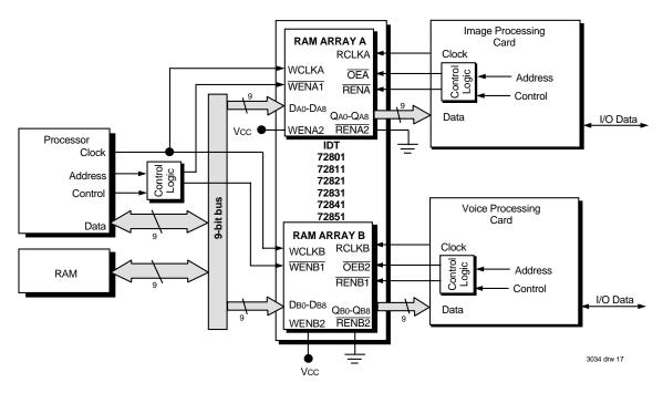
Figure 16. Block Diagram of Two Priority Configuration
