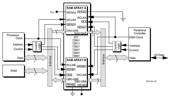
Figure 17. Block Diagram of Bidirectional Configuration
