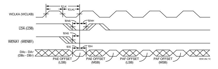
Figure 12. Write Offset Register Timing
