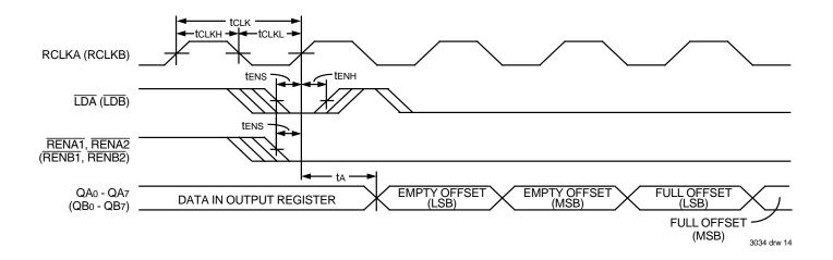
Figure 13. Read Offset Register Timing
