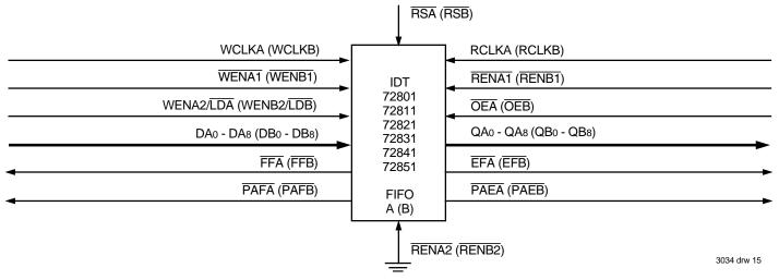
Figure 14. Block Diagram of One of the IDT72801/72811/72821/72831/72841/72851's two FIFOs configured as a single device
