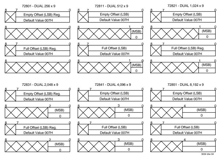
Figure 3. Offset Register Formats and Default Values for the A and B FIFOs
