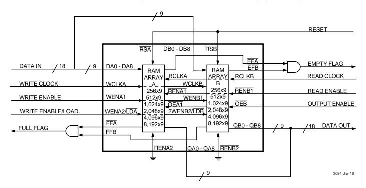
Figure 15. Block diagram of the two FIFOs contained in one IDT72801/72811/72821/72831/72841/72851 configured for an 18-bit width-expansion
