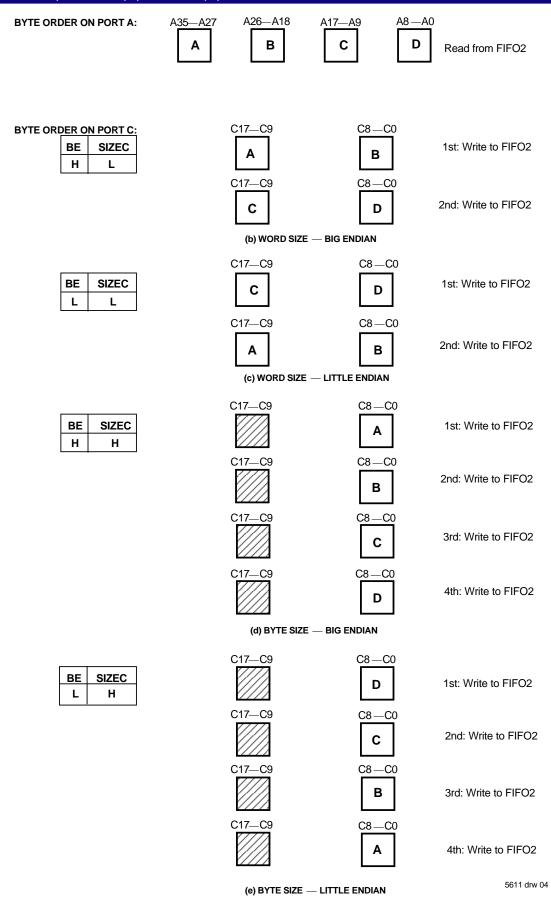
Figure 3. Port C Bus Sizing
