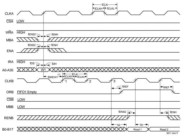
Figure 16. ORB Flag Timing and First Data Word Fall Through when FIFO1 is Empty (FWFT Mode)
