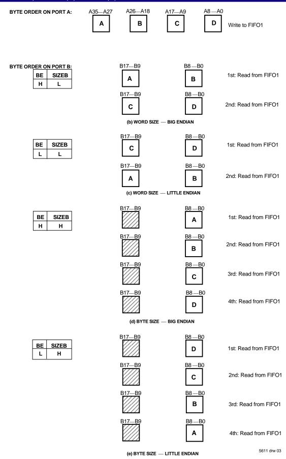
Figure 2. Port B Bus Sizing
