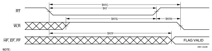
1.  $\overline{\text{EF}}$ ,  $\overline{\text{FF}}$  and  $\overline{\text{HF}}$  may change status during Retransmit, but flags will be valid at trtc.
