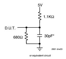
Figure 1. Output Load
