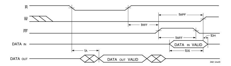
Figure 18. Write Data Flow-Through Mode
