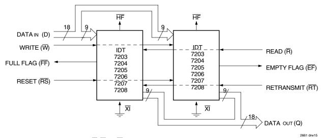
Flag detection is accomplished by monitoring the FF, EF and HF signals on either (any) device used in the width expansion configuration.
