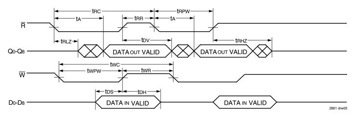
Figure 3. Asynchronous Write and Read Operation
