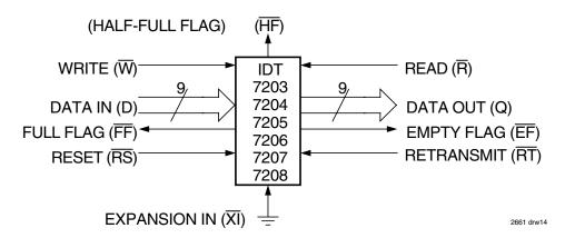
Figure 12. Block Diagram of 2,048 x 9, 4,096 x 9, 8,192 x 9, 16,384 x 9, 32,768 x 9, 65,536 x 9 FIFO Used in Single Device Mode
