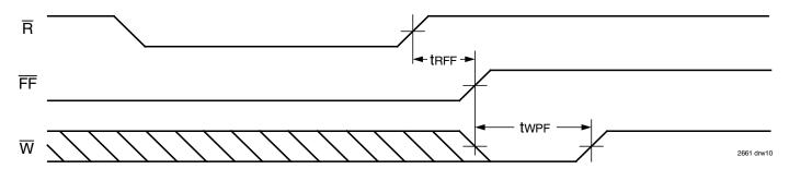
Figure 8. Minimum Timing for a Full Flag Coincident Write Pulse.
