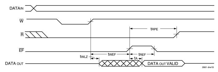
Figure 17. Read Data Flow-Through Mode
