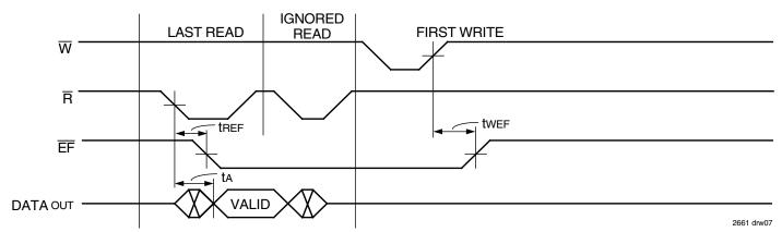
Figure 5. Empty Flag Timing From Last Read to First Write
