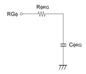
Reset gate clock equivalent circuit
