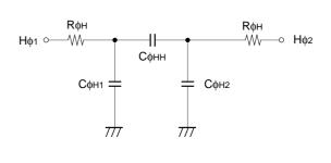
Vertical transfer clock equivalent circuit
