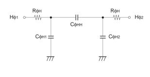
Vertical transfer clock equivalent circuit
