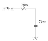
Reset gate clock equivalent circuit
