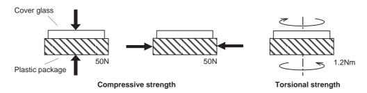
b) If a load is applied to the entire surface by a hard component, bending stress may be generated and the package may fracture, etc., depending on the flatness of the bottom of the package. Therefore, for installation, use either an elastic load, such as a spring plate, or an adhesive.
