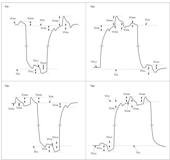
$V_{VH} = (V_{VH1} + V_{VH2})/2$
