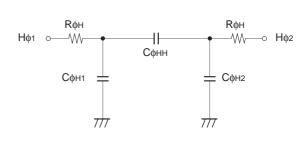
Vertical transfer clock equivalent circuit
