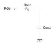
Reset gate clock equivalent circuit
