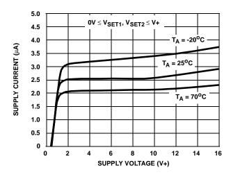
FIGURE 6. SUPPLY CURRENT AS A FUNCTION OF SUPPLY VOLTAGE
