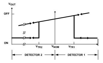
FIGURE 9B. TRANSFER CHARACTERISTICS FIGURE 9. SIMPLE THRESHOLD DETECTOR
