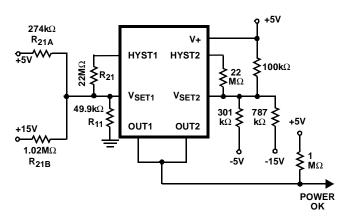
FIGURE 13. MULTIPLE SUPPLY FAULT MONITOR
