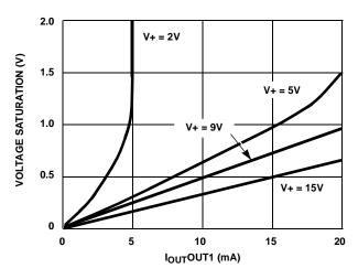
FIGURE 1. OUT1 SATURATION VOLTAGE AS A FUNCTION OF OUTPUT CURRENT
