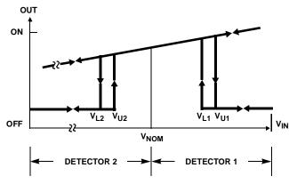
FIGURE 10B. TRANSFER CHARACTERISTICS
