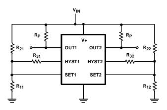
FIGURE 11. AN ALTERNATIVE HYSTERESIS CIRCUIT
