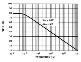
FIGURE 4. NPUT POWER SUPPLY REJECTION RATIO
