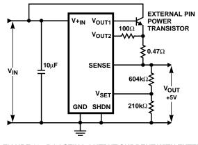
FIGURE 10. BOOSTING OUTPUT CURRENT WITH EXTERNAL TRANSISTOR
