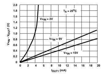
FIGURE 2. V<sub>OUT1</sub> INPUT-OUTPUT DIFFERENTIAL vs OUTPUT CURRENT
