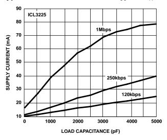
FIGURE 17. SUPPLY CURRENT VS LOAD CAPACITANCE WHEN TRANSMITTING DATA
