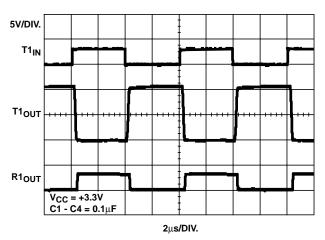
FIGURE 13. LOOPBACK TEST AT 250kbps (C<sub>L</sub> = 1000pF)
