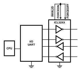
FIGURE 9. CONNECTIONS FOR AUTOMATIC POWERDOWN
