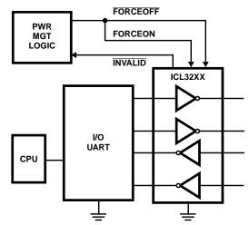
FIGURE 4. CONNECTIONS FOR MANUAL POWERDOWN
