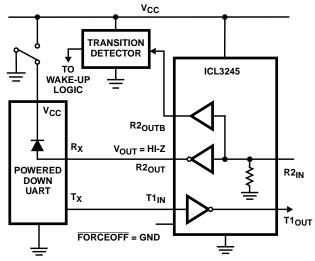
FIGURE 3. DISABLED RECEIVERS PREVENT POWER DRAIN
