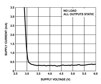
FIGURE 20. SUPPLY CURRENT vs SUPPLY VOLTAGE
