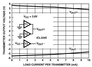
FIGURE 11. TRANSMITTER OUTPUT VOLTAGE vs LOAD
