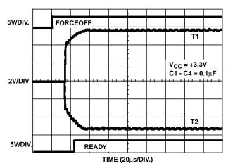
FIGURE 10. TRANSMITTER OUTPUTS WHEN EXITING POWERDOWN
