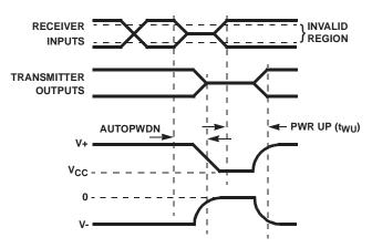
FIGURE 5. AUTOMATIC POWERDOWN TIMING DIAGRAM
