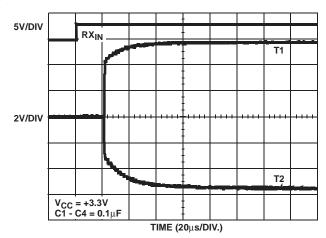
FIGURE 6. TRANSMITTER OUTPUTS WHEN EXITING POWERDOWN (ICL3217ONLY)
