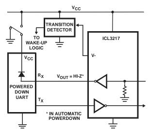
FIGURE 3. DISABLED RECEIVERS PREVENT POWER DRAIN
