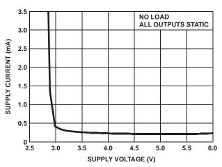
FIGURE 13. SUPPLY CURRENT vs SUPPLY VOLTAGE
