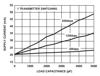
FIGURE 12. SUPPLY CURRENT VS LOAD CAPACITANCE
