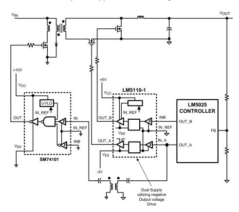
Figure 15. Simplified Application Block Diagram
