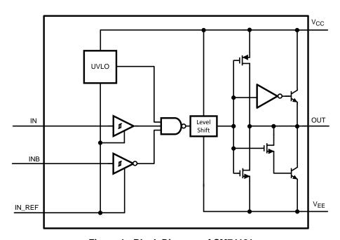
Figure 1. Block Diagram of SM74101
