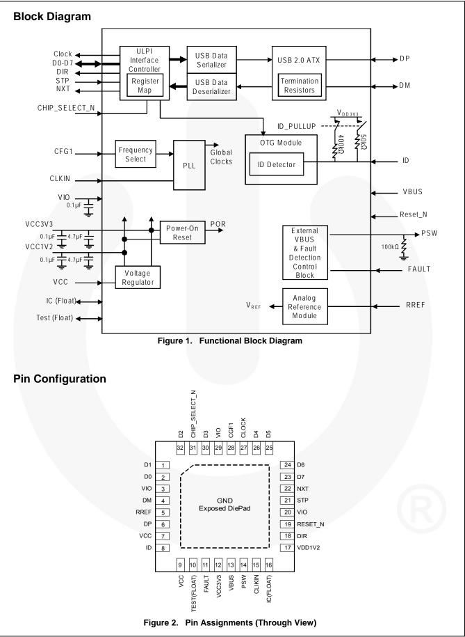
FUSB2805 — USB2.0 High-Speed OTG Transceiver with ULPI Interface
