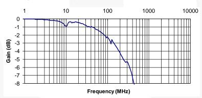
Figure 6. Bandwidth  $V_{CC} = 3.3 \text{ V}, C_L = 0 \text{ pF}$
