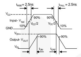
Figure 12. Turn-On / Turn-Off Waveforms
