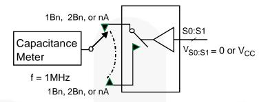
Figure 18. Channel Off Capacitance
