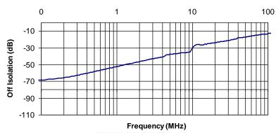
Figure 4. Off Isolation  $V_{CC} = 3.3 \text{ V,C}_L = 0 \text{ pF}$
