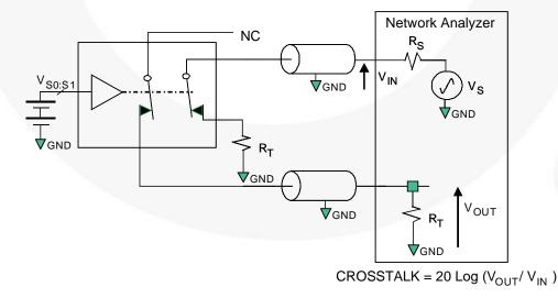
Figure 17. Non-Adjacent Channel-to-Channel Crosstalk
