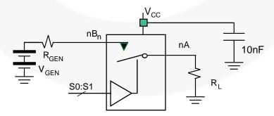
Figure 20. Total Harmonic Distortion
