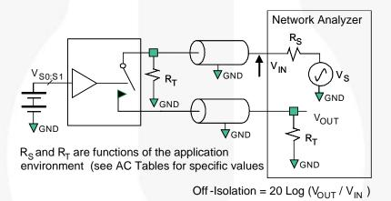
Figure 16. Channel Off Isolation
