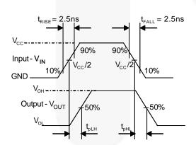
Figure 13. Switch Propagation Delay Waveforms
