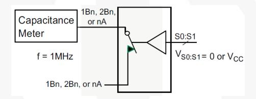
Figure 19. Channel On Capacitance
