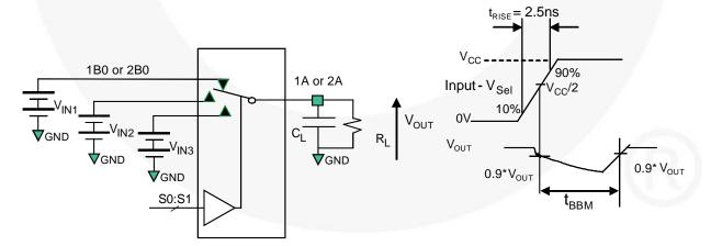
$R_L$  and  $C_L$  are functions of the application environment (see AC Tables for specific values)  $C_L$  includes test fixture and stray capacitance
