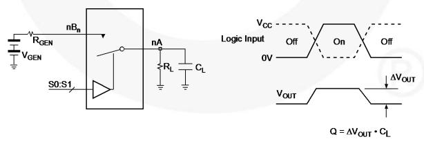
Figure 14. Charge Injection Test
