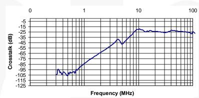
Figure 5. Non-Adjacent Crosstalk V<sub>CC</sub> = 3.3 V,C<sub>L</sub> = 0 pF
