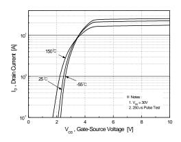
Figure 2. Transfer Characteristics
