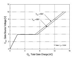
Figure 6. Gate Charge Characteristics
