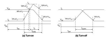
Fig. 4. Switching Time Definition
