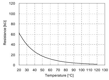
Fig. 9. R-T Curve of the Built-in Thermistor
