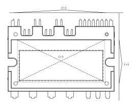
Fig. 5. Flatness Measurement Position
