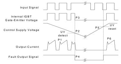
P1: Normal operation - IGBT ON and conducting current
